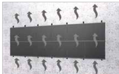
Very good rear ventilation of the modules
